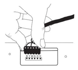
Terminal Connector Removal and Replacement
